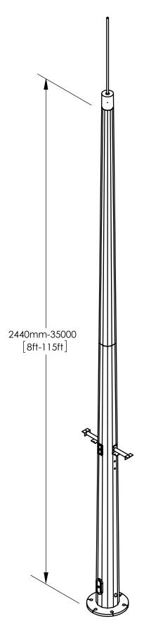
LIGHTNING PROTECTION MAST (roof top/A-Frame mount) 8 FT. to (high mast) 115 FT.
